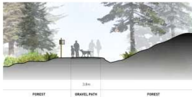
3 3.0M GRANULAR PATHWAY ON SLOPE Scale: 1:75
