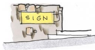
Signs Recessed in Stone Walls
