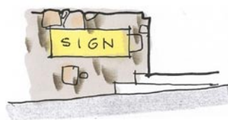
Signs Recessed in Stone Walls
